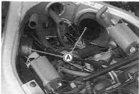
A. Air Intake Ducts
