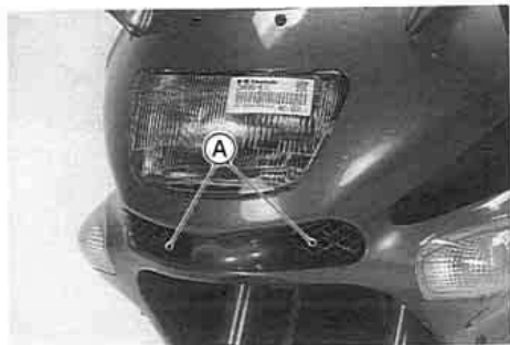
A. Air Cleaner Intakes
